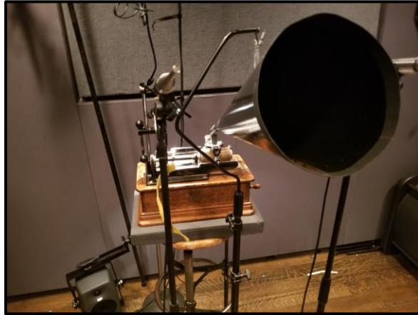
Figure 11. The Edison Home Phonograph and the black metal phonograph horn replica used during data collection.
